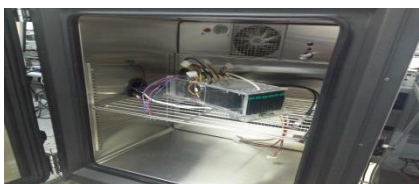
Fig. 5. Drive assembly with wind tunnel placed in thermal chamber
